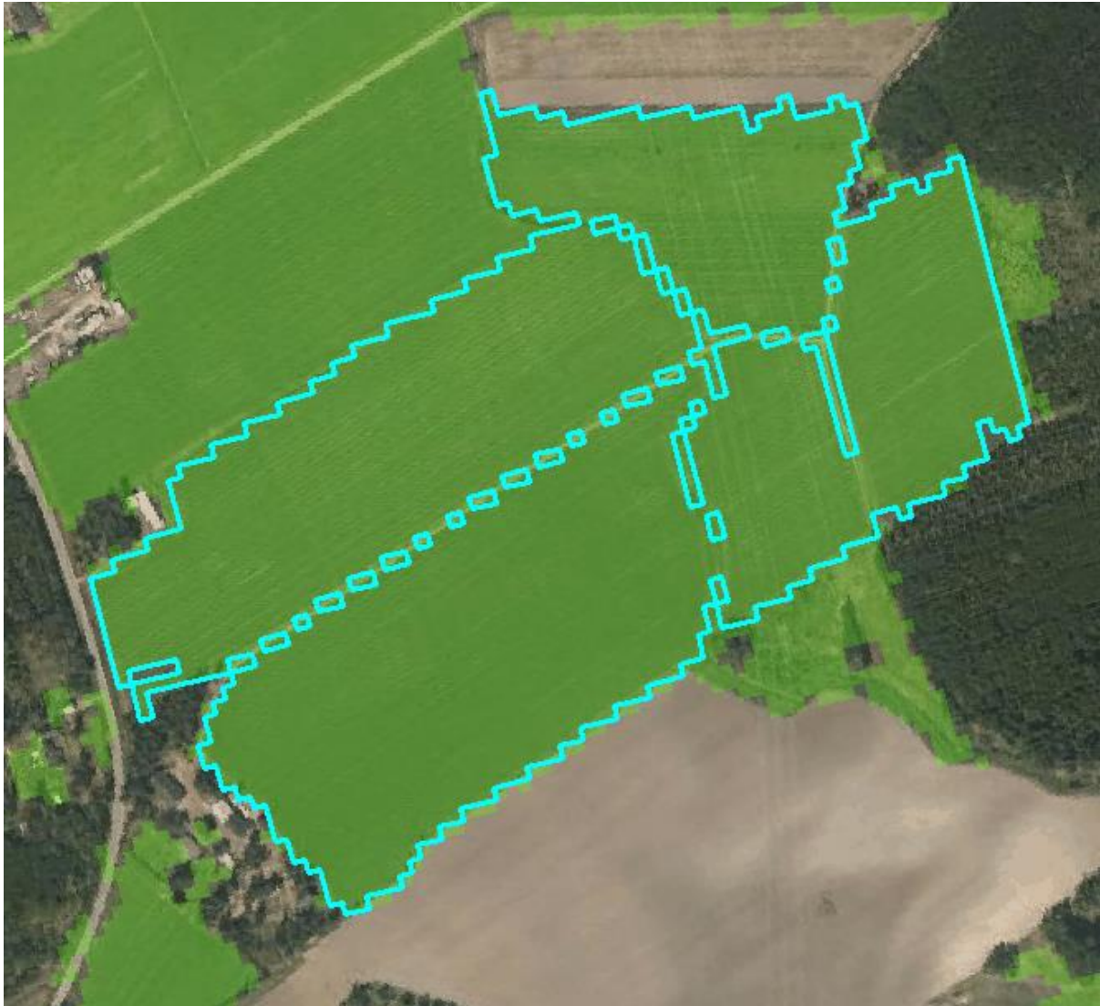
Figure 8. Commission errors in a blackcurrant plantation. The turquoise polygon is the contradicting area derived from the GIS comparison of in-situ data and the HRL GRA18. GRA18 data is presented with light green. SAMPLE_ID 197, scale 1:5000, coordinates (ETRS_1989_LAEA) E: 5217437 N: 4292930. Ortho photo reference year 2018.
